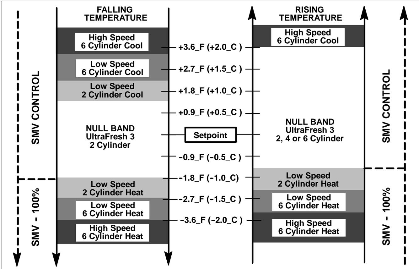
Figure 4-1. Continuous Run Temperature Control Operating Sequence - Perishable Range
