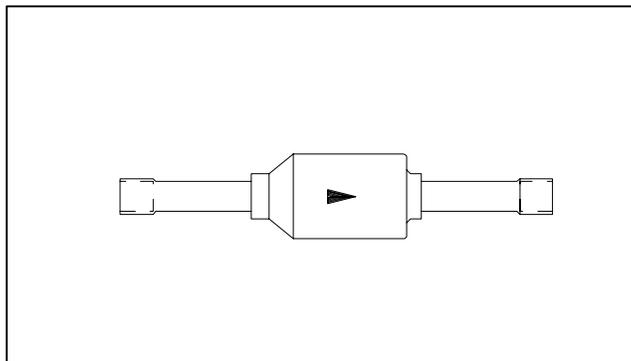
**Figure 8-22. Hot Gas Check Valve (Non-Serviceable)**
