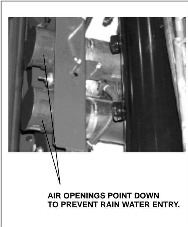
**Figure 3-5. AutoFresh in Closed Position**
