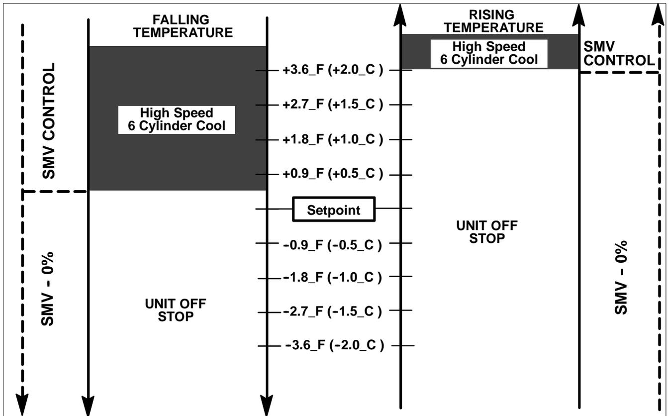
Figure 4-4. Start-Stop - Temperature Control Operating Sequence - Frozen Range
