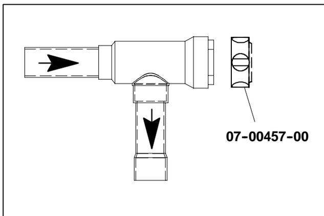
**Figure 8-21. Discharge Check Valve (Non-Serviceable)
