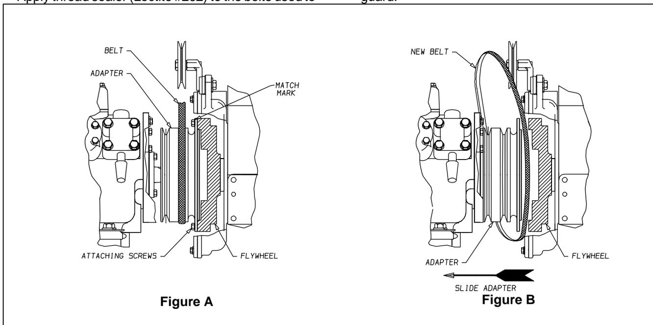
Figure 8-11. Removing V-Belt from Engine Adapter Drive Sheave
