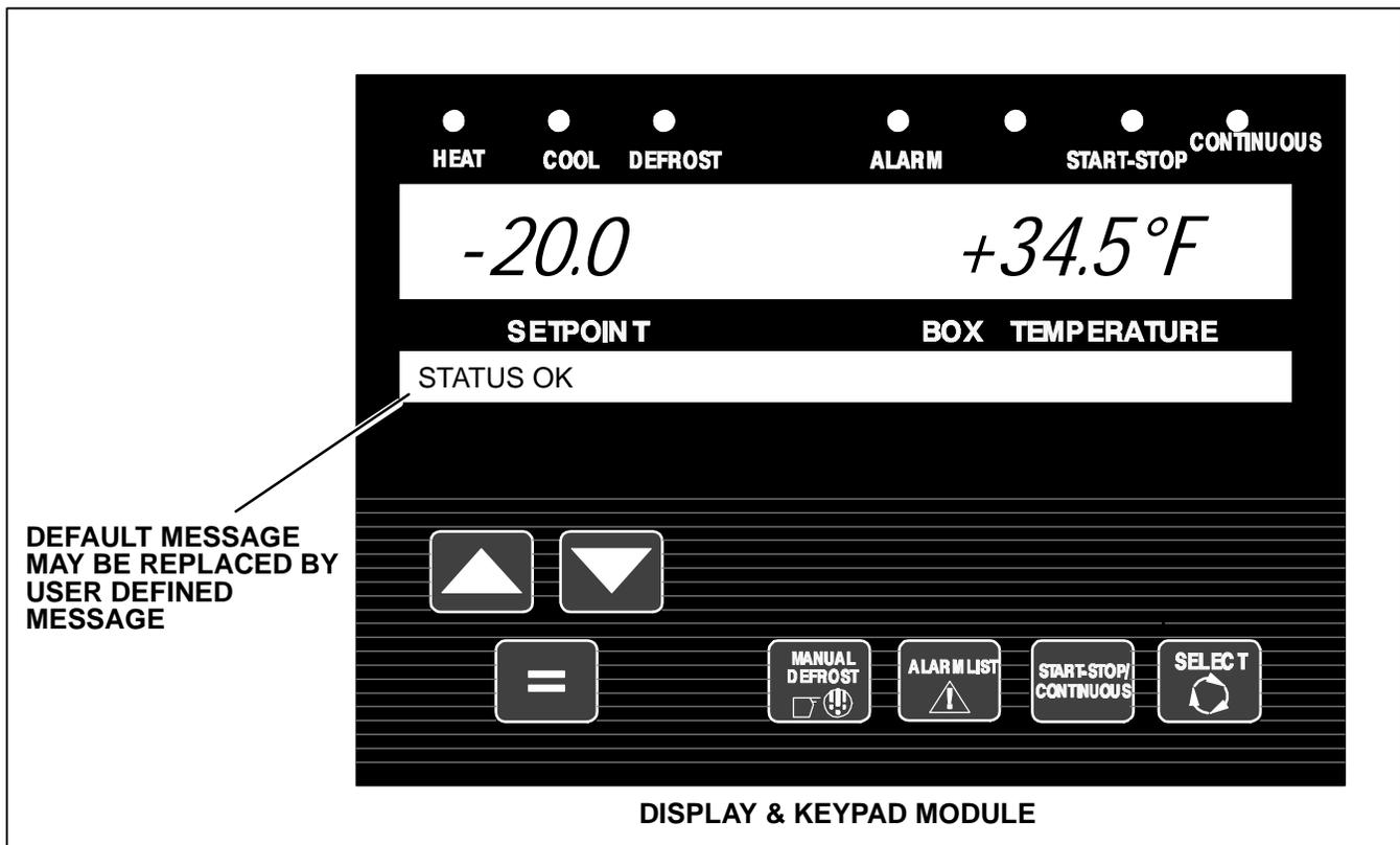
The Display & Keypad Module is located for operator access at the lower roadside corner of the unit.
