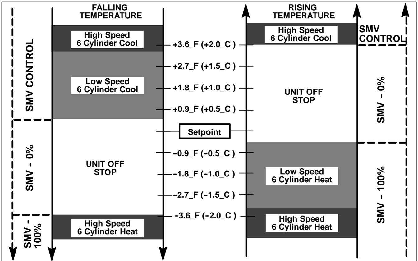
Figure 4-3. Start-Stop - Temperature Control Operating Sequence - Perishable Range
