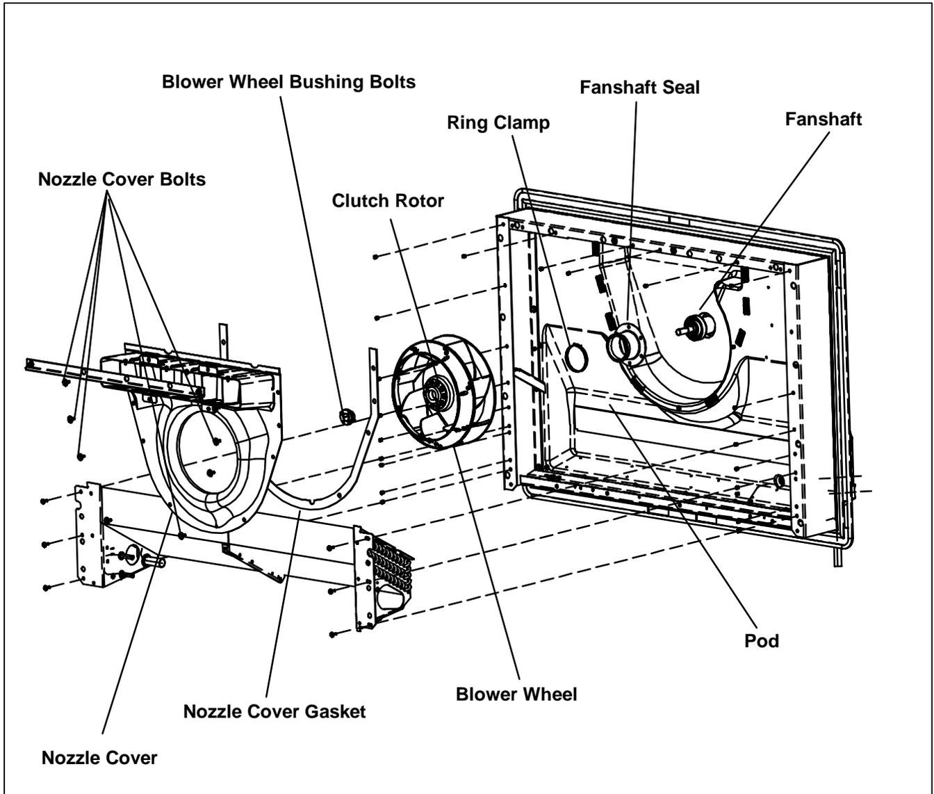
Figure 8-13. Blower Wheel And Nozzle Cover Assembly
