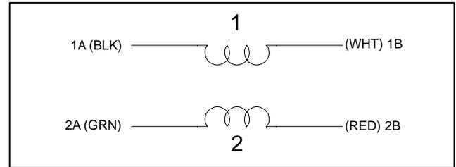
**Figure 8-29. SMV Coil (Bi-Polar Design)**
