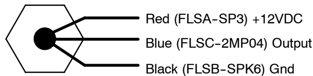
Figure 8-4. Fuel Level Switch Wiring
